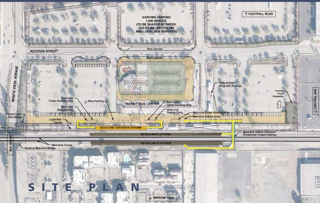
The Montclair station will be located at the Montclair TransCenter, just east of Monte Vista Avenue and north of Arrow Highway. The Gold Line station will be a center platform station, with light rail tracks on either side (one for westbound and one for eastbound trains) and will be located to the north of the existing Metrolink platforms. A connection will be built between the Gold Line and Metrolink platforms via the existing pedestrian tunnel to facilitate pedestrian movement between systems.
