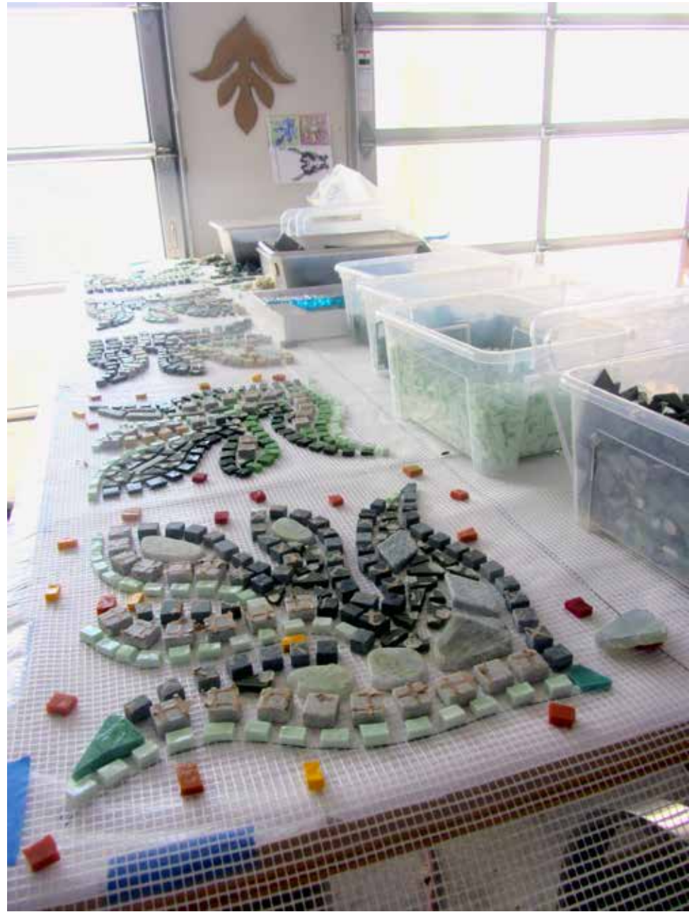
The process of creating and casting LithoMosaic pavers requires detailed handwork. Each paver is an individual composition of glass tiles, natural stone, and texture.
